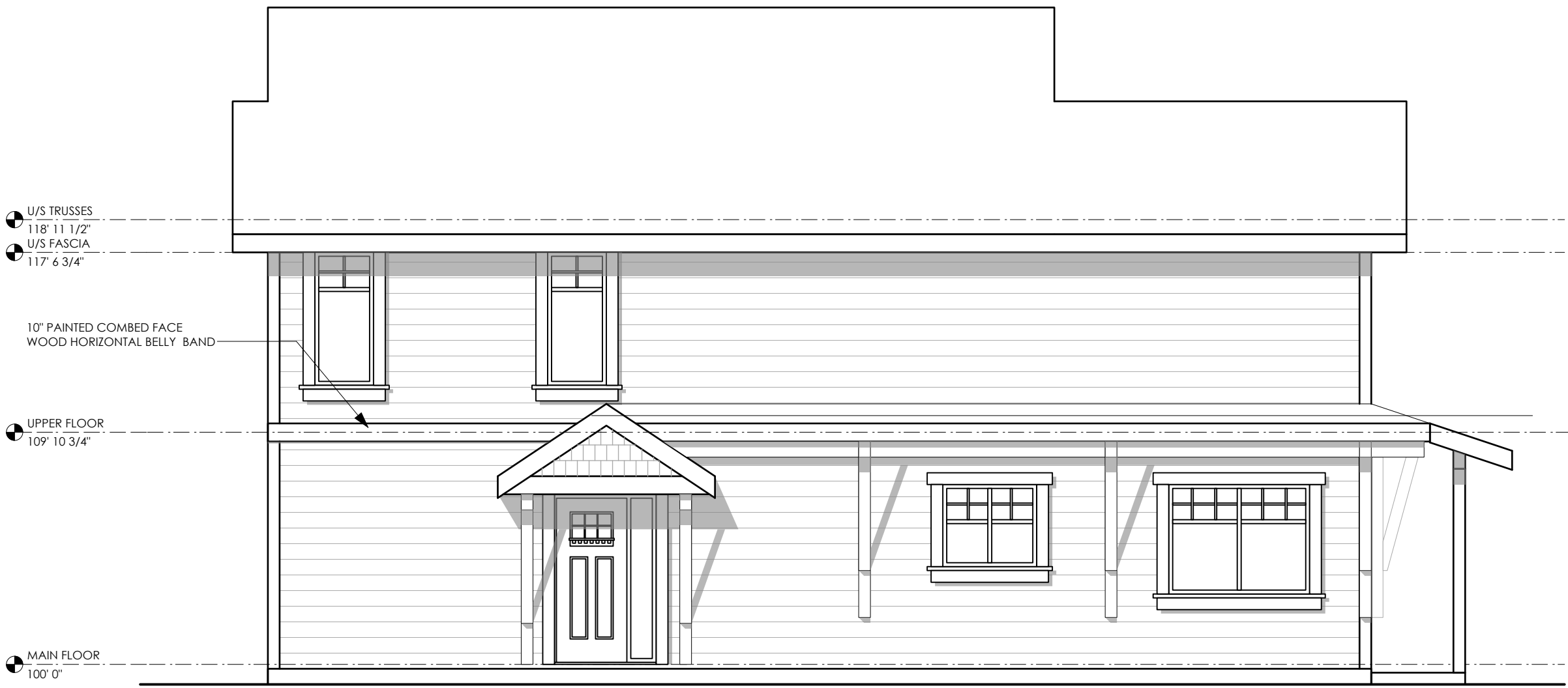
5 South Elevation PR2 3/16" = 1'-0"
